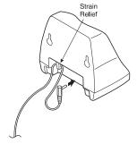
3. Place the Charging Unit on the posts of the wall screws and push down until it is firmly seated.
